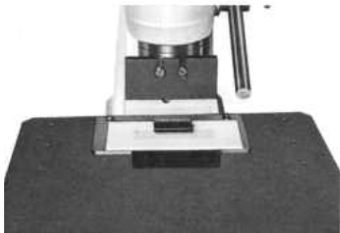
3. Set insertion support plate in place by butting it against Mini-Press platform.
